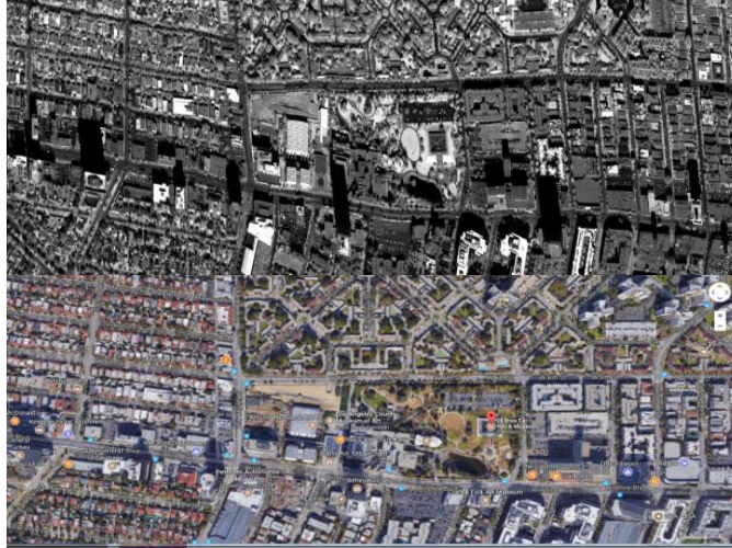
Fig. 1. SWIR hyperspectral band average (top) of a multi-block urban region of Los Angeles, USA, next to its correspondent Google Map image (bottom). The area includes live vegetation (tree, grass) and manmade structures (e.g., roads, parking lots, high buildings, houses). By visual inspection one can notice the spatial feature similarities between the SWIR and Visible color images, which we plan on automatically extracting and exploring for image registration.
