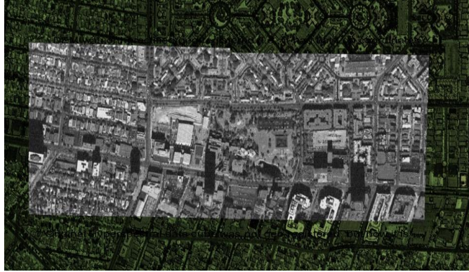
Fig. 4. Successful registration between the SWIR band image (embedded gray scale image in the center) and a spatial location within the DEM's orthophoto (larger image).
